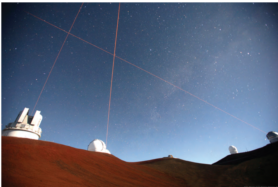
FIGURE 7.6 Three laser adaptive optics systems operating on Mauna Kea. SOURCE: © Subaru Telescope, National Astronomical Observatory of Japan. All rights reserved. Reprinted with permission.
